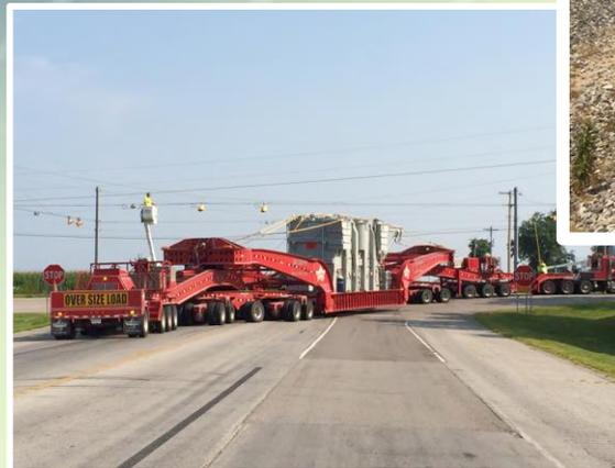
HLI received this 378,936 power transformer secured to a railcar in Eagle Pass, TX. With GPS and impact recorder installed, the unit traversed the tracks from Texas to a rail siding in Hagerstown, IN. It arrived in Hagerstown safely and was promptly lifted off the railcar by a gantry system and transloaded onto a dual lane trailer.
