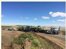
This 240,000 lbs transformer entered the United States on rail in Eagle Pass, TX. HLI installed an impact recorder and GPS on the unit to track the unit on its long journey north. 2,527 rail miles later, the transformer arrived at a rail siding in Dayton, WA. At the rail spur, the rigging crew jacked up the transformer and moved it across slides to a specialized dual lane transport trailer for the haul to site.
