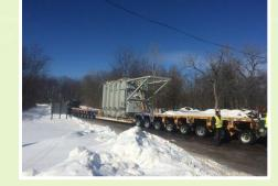
This 296,211 lb transformer set out on its journey from Eagle Pass, TX equipped with a GPS tracker and impact recorder. It traveled by rail through the heart of the country to a siding in Bedford, OH. The unit arrived safely at the spur where the rigging crew set to work. They jacked the transformer up and maneuvered slide beams underneath it. Slowly and deliberately, the team relocated the unit onto an 8 deck 8 Goldhofer trailer.
