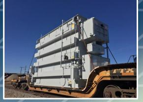
HLI received this 201,800 lbs transformer loaded and secured on a railcar in Waukesha, WI. After a mechanical inspection, HLI's team railed the unit 1,394 miles south to a rail siding in Big Spring, TX. At the rail spur, HLI employed an all-terrain crane to lift the transformer off the railcar and place it onto a specialized girder transport trailer for the subsequent haul to site.
