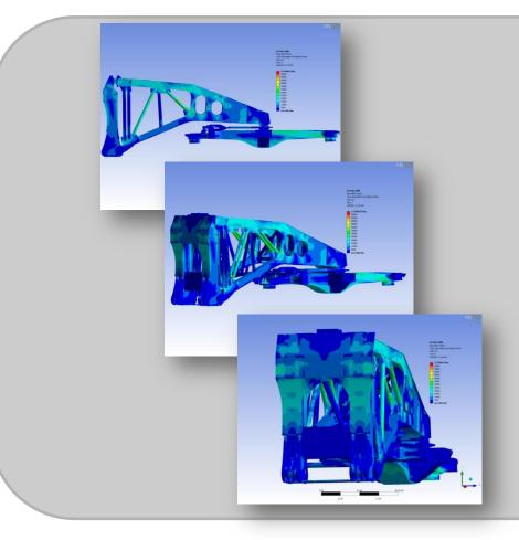
Red or Orange Coloration Denote Areas of High Stress. As you can see, CCRX 40010 handles its maximum gross load with ease. No expense was spared to provide the safest, most efficient Schnabel Railcar
