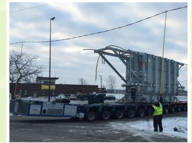
The transformer entered the United States on a railcar in Eagle Pass, TX. HLI then coordinated the delivery to a rail siding in Toledo, OH, where it would be transferred to a Goldhofer, for the final portion of the delivery to the substation. Once arrived at the rail siding, HLI's crew set to work, unleashing the transformer from the railcar, and preparing the slide, to place it on to the Goldhofer.
